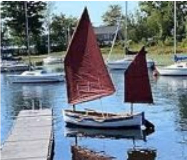
coast of Maine in the 19th & early 20th centuries. I can rig this Tender with a single lug sail, or a lug-rigged cat yawl with two mast. It is a easy set up at the beach rigging the sails. I can have the boat off the trailer, rigged, and sailing in 15 minutes! I started this project in April and finished it in July. About 250 hours of dedicated work. During this pandemic I was able to focus on this project. I didn't think I would compete it so quickly. In a way it was like building a model ship.
